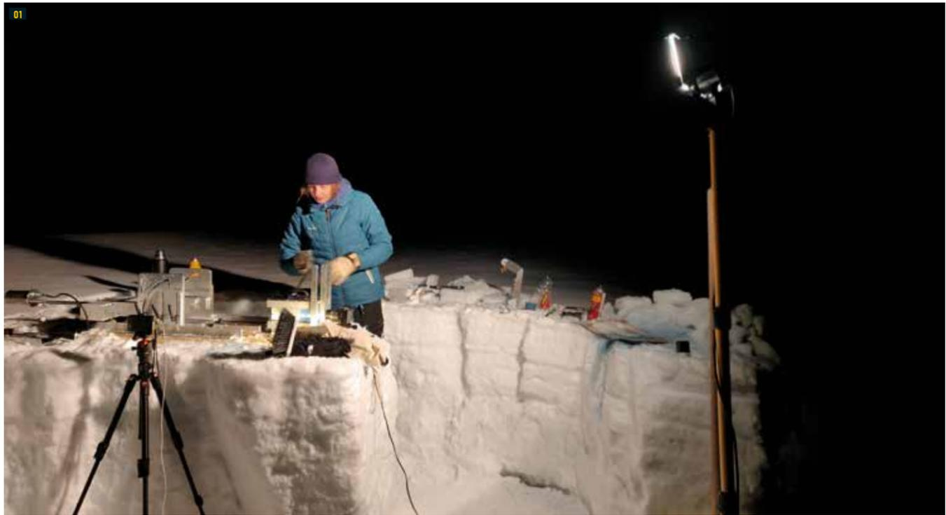
01 Testing a weak layer of buried surface hoar on 14 February 2024 above Davos, Switzerland. As the weather was warm and sunny, we had to perform our experiments at night to ensure our samples would not melt. (Photo: V. Adam) |
